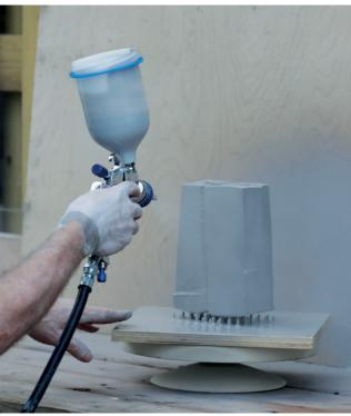
**24** Larger forms are glazed by spraying. I pour the glaze into the inside first, clean off any drips, then spray over the exterior. As I usually require a thick application of glaze, I build it up in layers, allowing each layer to dry before applying the next. Spraying each piece standing on a board of screws prevents a build-up of glaze around the base of the form.
