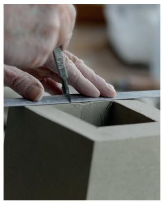
**12** After the clay blank is trued up, I focus on tidying up the interior of the vessel. Using a fine scalpel, I score a line around the opening. This gives me a guideline to cut back to.
