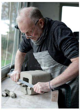
**11** Once the clay has reached the desired dryness, I begin the shaping process. The first stage involves shaving a slice off each side in order to square off faces and corners. The tool I have found best suited for this process is a blade from a woodworking planer thicknesser. As these large cuts often require significant force using an extremely sharp blade, considerable care is required at this stage.
