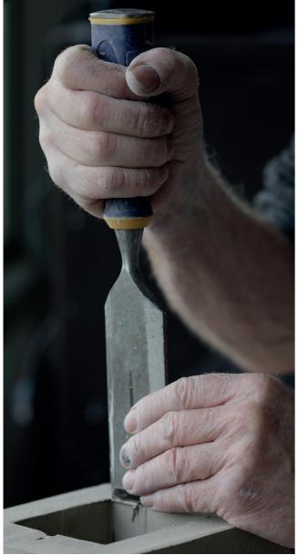
**13** Using a sharp woodworking chisel and the scalpel line as a cutting guide, I pare back each of the interior walls, carefully working my way around each side to produce an interior with crisp sides and edges.
